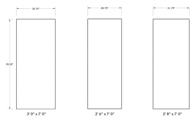
NOTE: BY REQUEST, DOOR HEIGHT COMES IN VARYING DIMENSIONS TO A MINIMUM OF 83". EXCESS WILL BE TAKEN FROM BOTTOM RAIL. ALL OTHER DIMENSIONS WILL REMAIN THE SAME.
